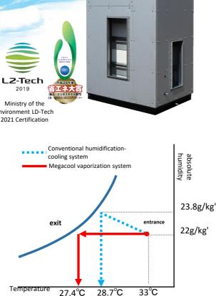
Air conditions Air supply side (Dry air): 33°C, 22 g/kg' Return air side (Wet air): 27°C, 10.5 g/kg'
